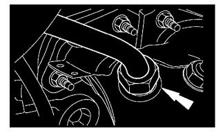
5. Disconnect the exhaust gas recirculation valve tube and remove it.
